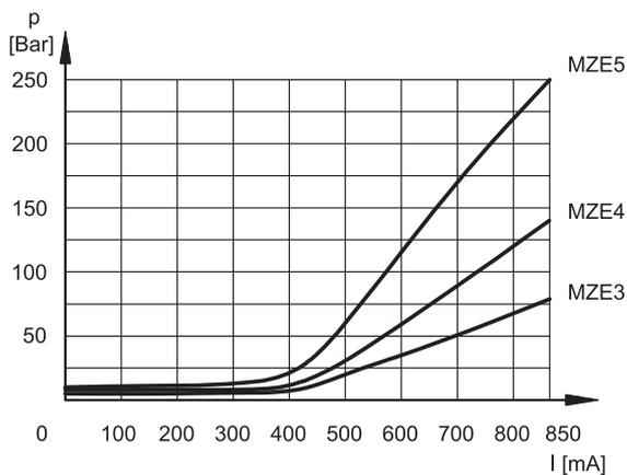
The curves have been obtained with closed users (without flow).
