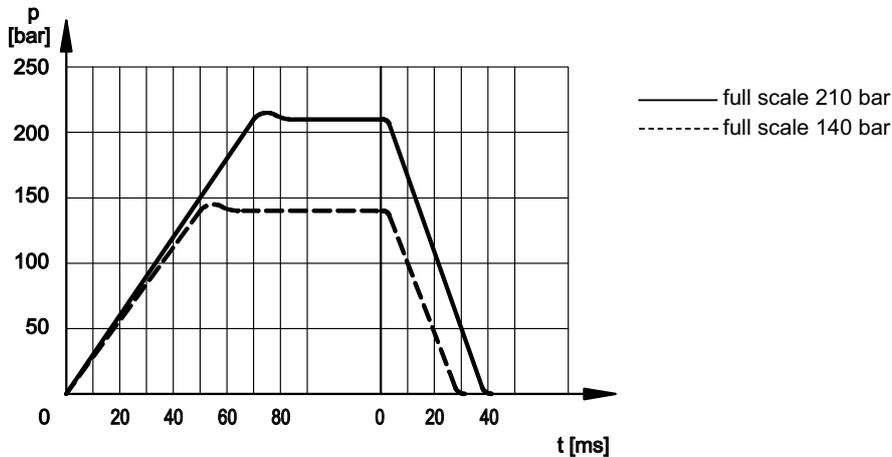
**NOTE:** Response times are obtained by using PRE25J valves with a full scale of 140 and 210 bar.
