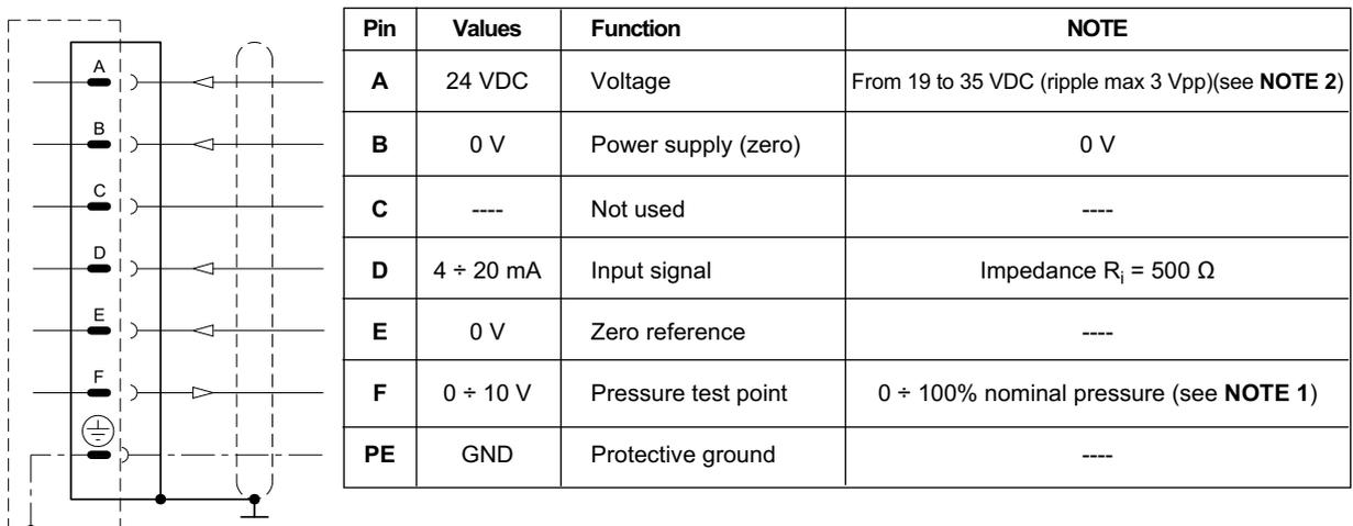
**NOTE for the wiring:** connections must be made via the 7-pin plug mounted on the amplifier. Recommended cable sizes are 0,75 mm<sup>2</sup> for cables up to 20m and 1,00 mm<sup>2</sup> for cables up to 40m, for power supply. The signal cables must be 0,50 mm<sup>2</sup>. A suitable cable would have 7 cores, a separate screen for the signal wires and an overall screen.
