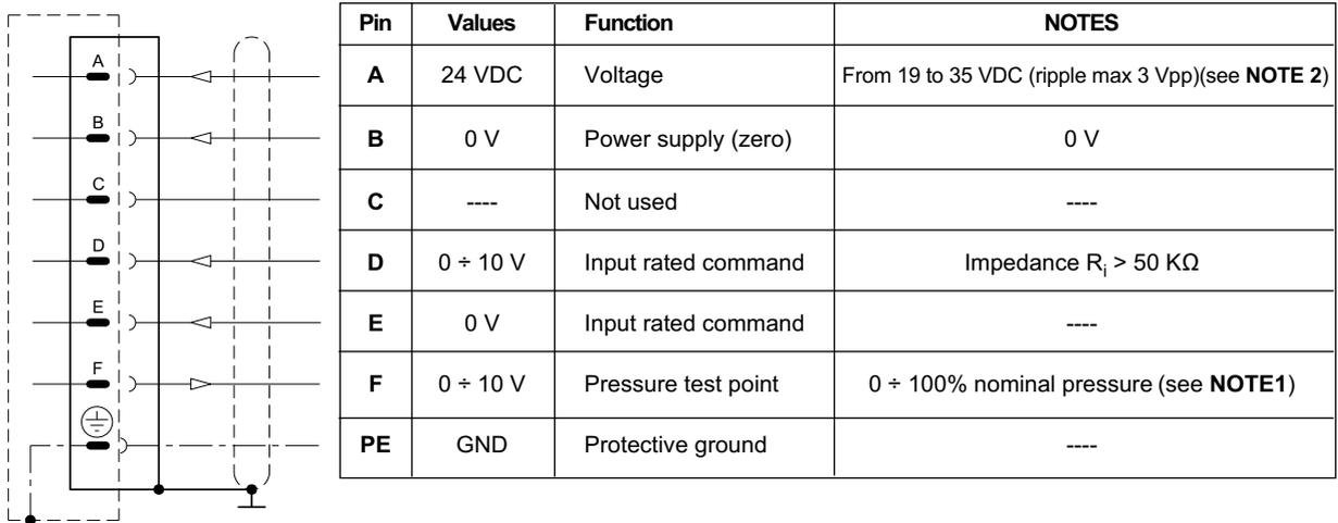
**NOTE:** If only one input signal is present, the pin B (0V power supply) and the pin E (0V reference signal) must be connected through a jumper and both connected to GND, electric panel side.
