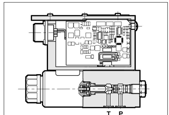
— The PRED3G valve is a direct operated pressure control valve with integrated electric proportional control and mounting interface in compliance with ISO 4401 (CETOP RP 121H) standards.
