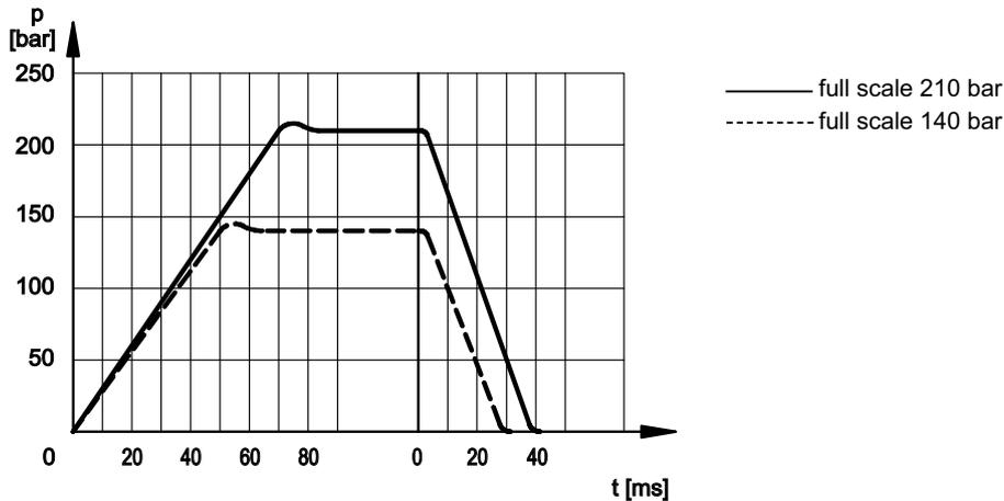
**NOTE:** Response times are obtained by using valves with a full scale of 140 and 210 bar, with an input flow rate of 2 l/min and a pressure oil volume of 0,5 lt. The response time is affected both by the flow rate and the oil volume in the pipework.
